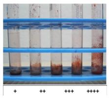
Figure 4. Tube biofilm formation
